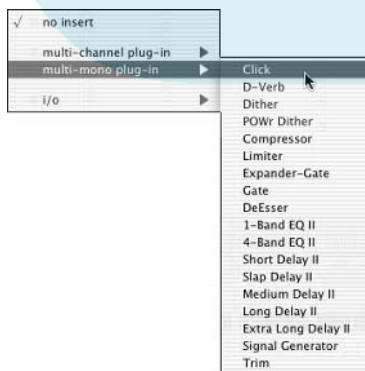
Figure 1-10: Choose the click plug-in from the Insert pop-up menu on the track's channel strip to play the click track.
